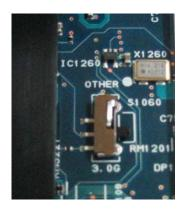
2. When a CPU other than 3.06GHz (2.53, 2.66, 2.80GHz) is used: Set the SLIDE SWITCH to the position of silk-printed "OTHER", which is on the CPU side of the system board.
